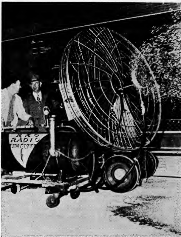
Fig. 18. Equipment for producing falling snow with foaming agents.
